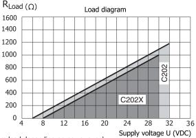
Maximum load depending on power supply Formula for the max. permissible output load for C202:  $R_{Load} = (U-6)/0.022$  Formula for the max. permissible output load for C202X:  $R_{Load} = (U-8)/0.022$
