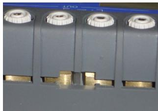
Connect your probes by simply pushing on the terminal top and insert wires of up to 3 mm or 10 AWG diameter and compensated thermocouple connectors.
