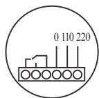
SA□□□A 110V/220VAC Relay output
