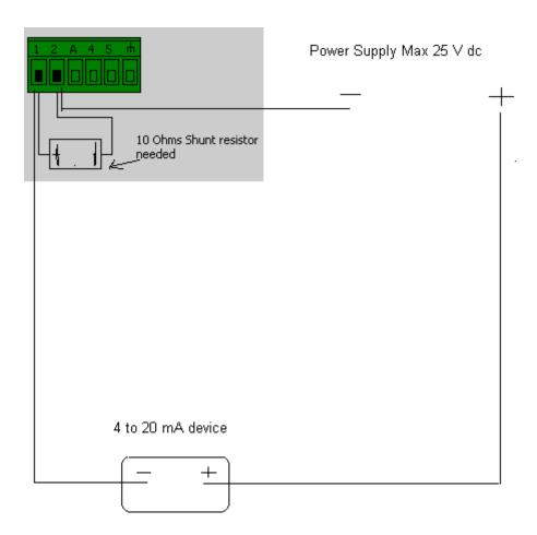
Sensors can be powered via the SQ2020/SQ2040 data logger if required maximum supply voltage is 18Vdc (supply volts) & total maximum current is 100mA.
