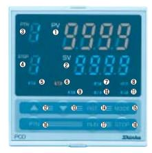
①PV display : Indicates Process variable (PV). During the setting mode, this
