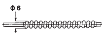
TYPE L5 - Capillary AISI 304 st.st. covered with zinc plated steel armour PVC coated TYPE L6 - Capillary AISI 304 st.st. covered with AISI 304 st.st. armour PVC coated TYPE L8 - Capillary AISI 316 st.st. covered with AISI 316 st.st. armour TYPE L9 - Capillary AISI 304 st.st. covered with AISI 304 st.st. armour
