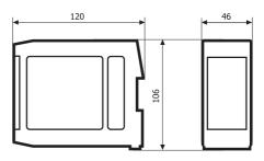
Measurements in mm
