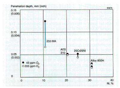
Figure 6. Testing for 400 h at 825°C (1515°F) in nitrogen containing 43 and 205 ppm  $\rm O_2$  , respectively.
