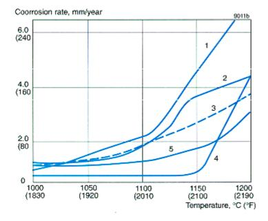
Figure 3. Oxidation in air during cyclic testing 5x24 h with cooling to room temperature every 24 h. Comparison of 253 MA with four other high-temperature materials.
