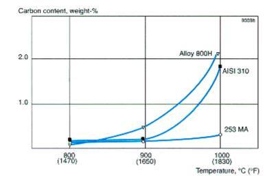
Figure 5. Carburisation of a cylindrical test piece at 0.5 mm (0.02 inch) distance from the surface after testing for 500 h at different temperatures in about 10% CH $_4$  + about 90% Ar + 0.5% O $_7$ .
